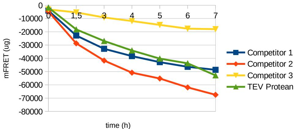
1. Image 2: Example graph of decreasing amount of FRET (ug) against time (hours) in measured samples. Fluorescence is decreasing into negative numbers after subtracting blank sample. The start (0 hours) correspond to 0 fluorescence upon subtraction of the background.
